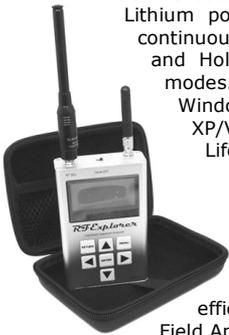
Pocket size and light weight, completely portable, solid aluminum metal case. 2 year warranty. Two separate inputs and three antennas supplied: a wideband telescopic antenna for all sub-GHz frequencies, a rubber duck 5.8 GHz and a whip helical for 2.4GHz band. Additional, specific band antennas may be needed to cover efficiently some of the frequencies supported. (Can also be used with Near Field Antenna on Page 79).
