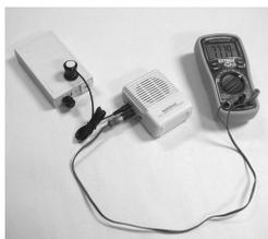
EarthSafe produces a measurable electromagnetic field. The frequency of this field can be varied from about 2 Hz to about 25 Hz. Using this kit, you can measure the
